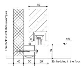
Installation situation: Door installation before laying the top flooring
